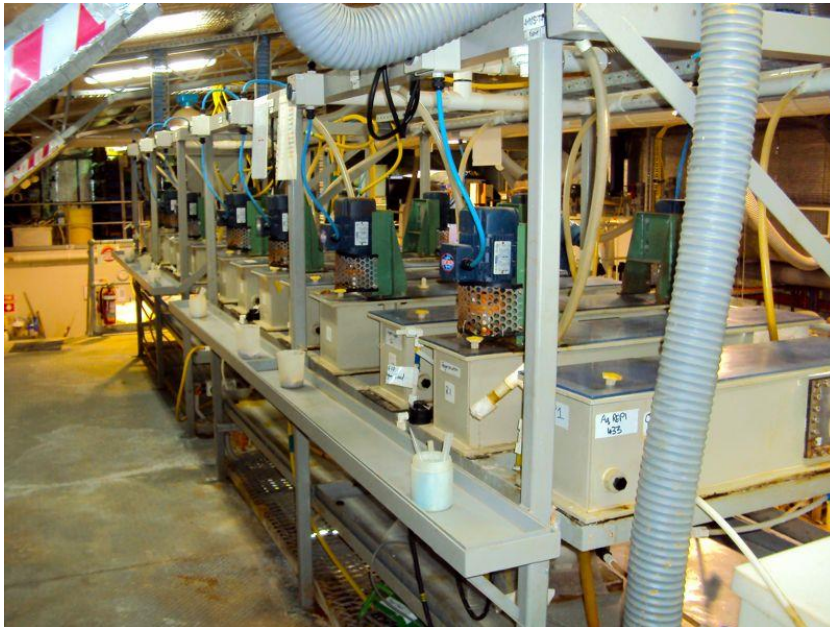
Figure 47 - Cellules SX en Australie (Alkane Resources demonstration plant, Dubbo project) source : www.techmetalsresearch.com
